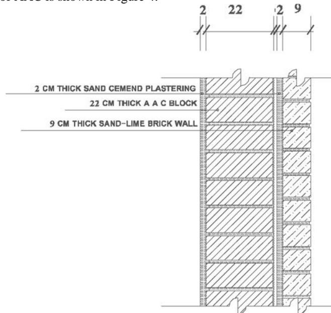
*Figure 4. AAC block wall.*
