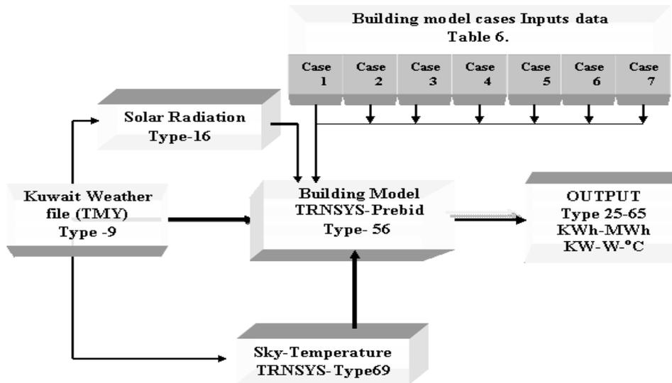
Figure 1. TRNSYS-System configuration and formative structure of the TRNSYS-Types used for the simulation of building cases thermal performance.
