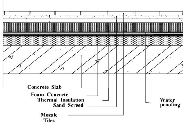
Figure 5. Detailed construction section of Kuwaiti flat roof
