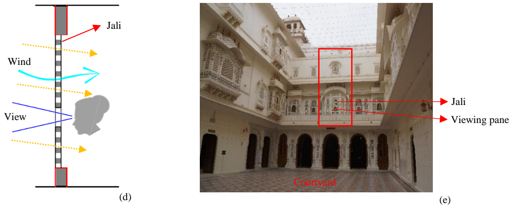
Figure 6. Openings (a) Small opening for visual connection, (b) near floor and roof for ventilation (c) Junagarh fort, Bikaner, Rajasthan, India (d) ventilation and visual connectivity with jali and (e) Junagarh fort, Bikaner, Rajasthan, India. (Source: Clicked by author)
