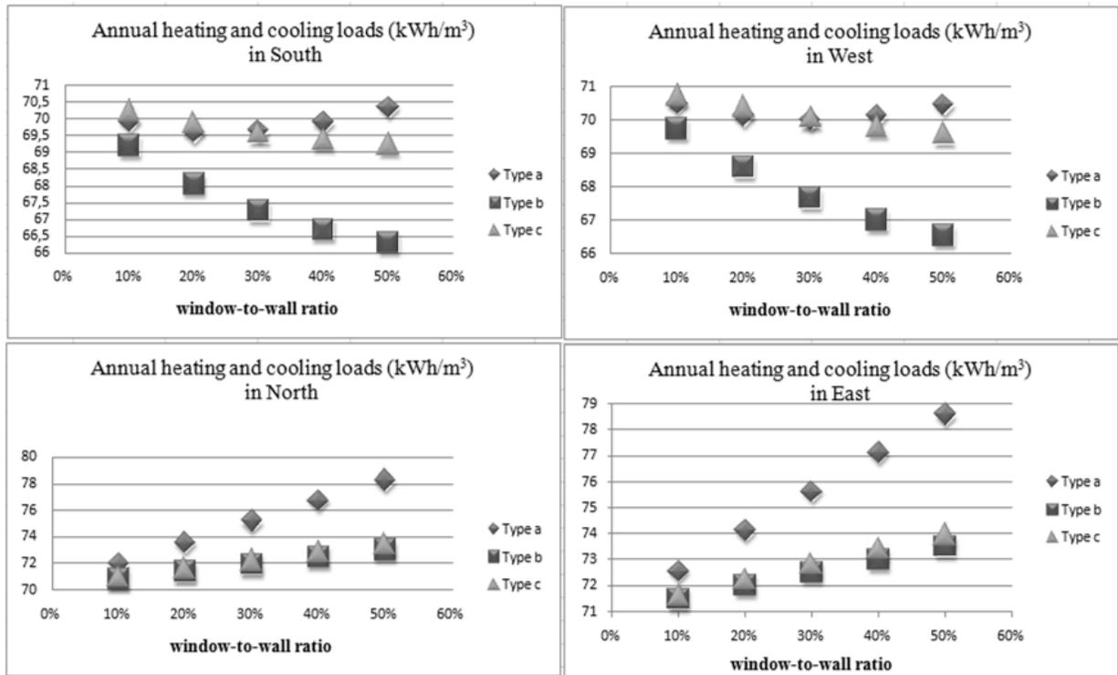
Figure 6. Annual Heating and cooling loads for different orientations when varying the glazing size (WWR).
