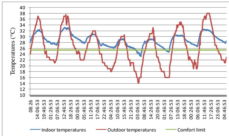
Figure 4. The variation of air temperature in the monitored office from 03 to 10 august 2014
