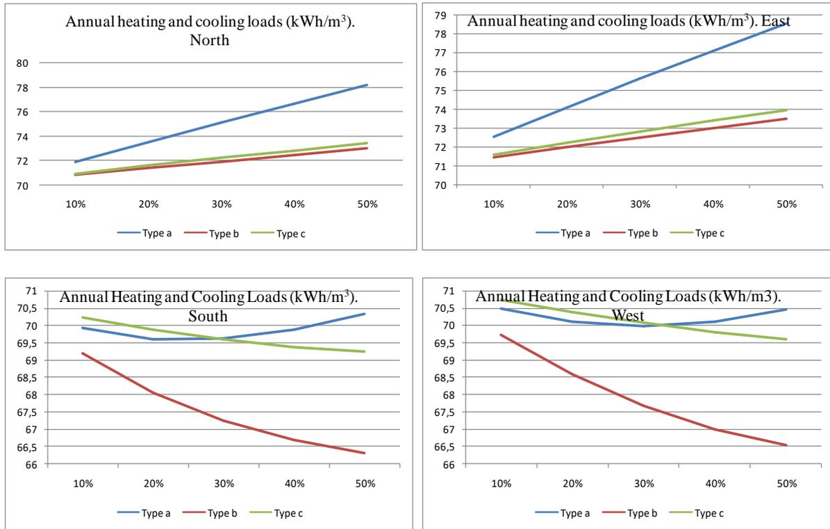
Figure 8. Heating and cooling energy demand for glazing Type (a), Type (b), and Type (c) for all the studied orientations.
