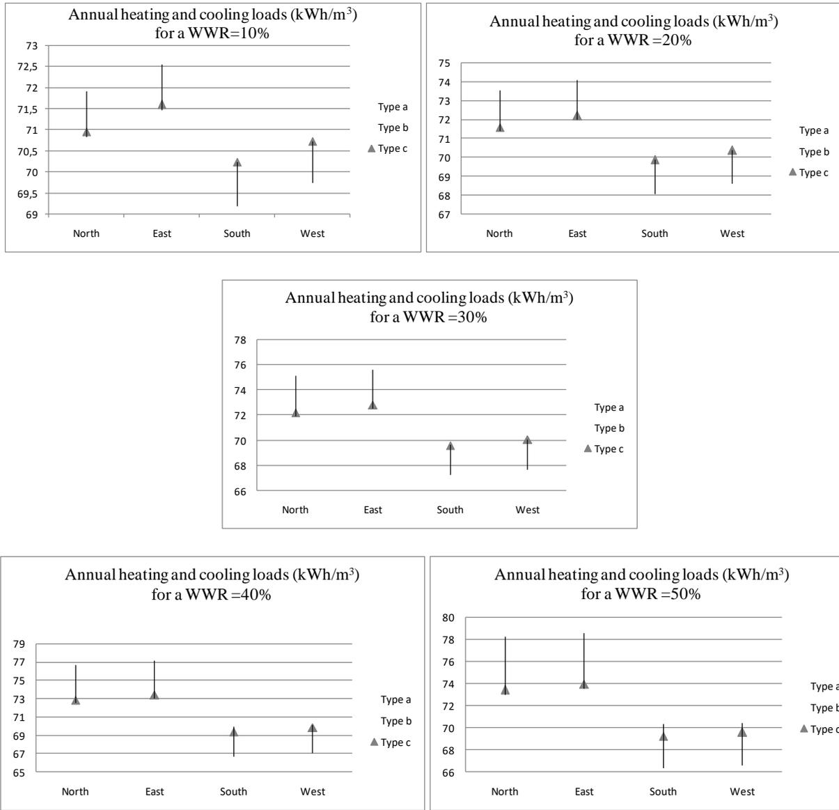
Figure 7. The effect of orientation on heating and cooling load.
