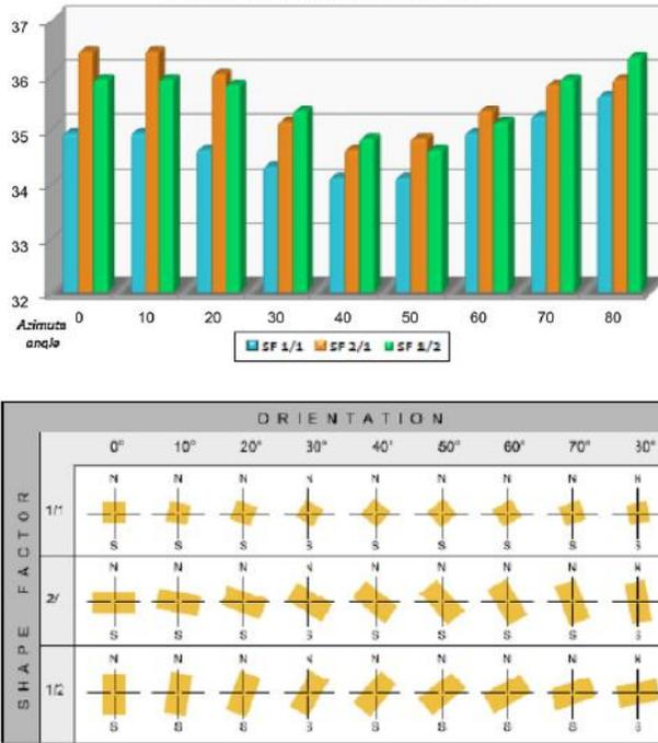
Figure 2. Heating energy saving, depending on shape and orientation (Aksoy and Inalli, 2006)
