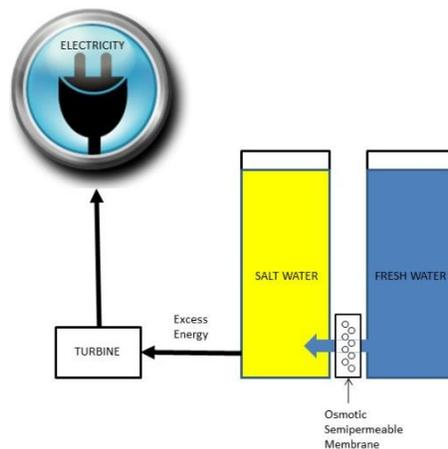
Figure 9. Osmotic pressure difference sea water and fresh water creates Blue Energy
