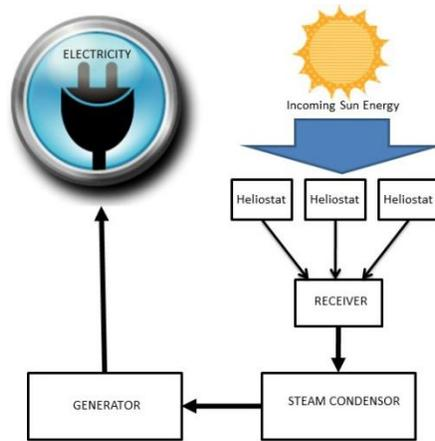
Figure 6. Power tower plant
