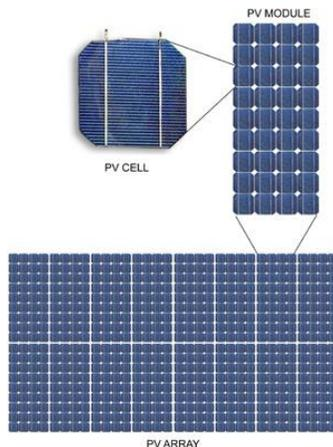
Figure 7. Photovoltaic systems
