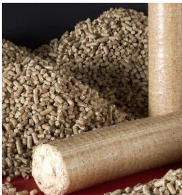
Figure 2. Wood pellets made from compacted sawdust have high combustion efficiency and are used as bio-fuel. (Courtesy of Scion)
